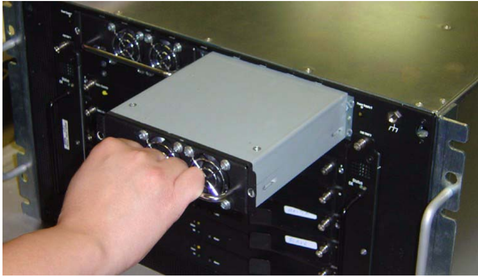
Figure 3-3: Pulling the Power Supply Module from the Bay
